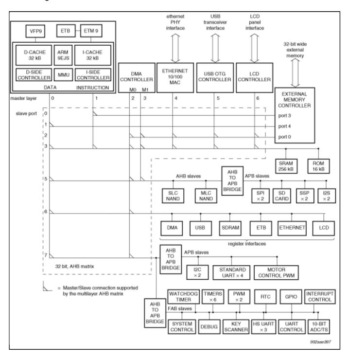
View additional information for Arm926EJ-S™ with 128 kB SRAM, USB High-speed OTG, SD/MMC, NAND flash controller.
