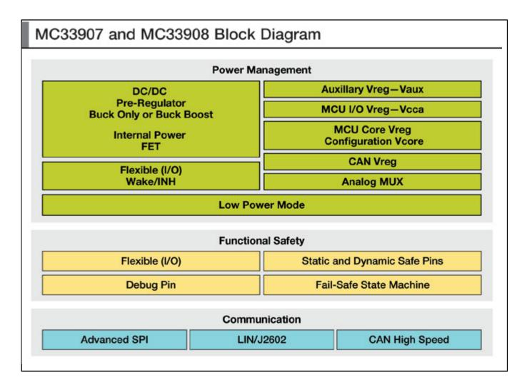
View additional information for Safe System Basis Chip with Buck and Boost DC/DC up to 1.5 A on Vcore.
