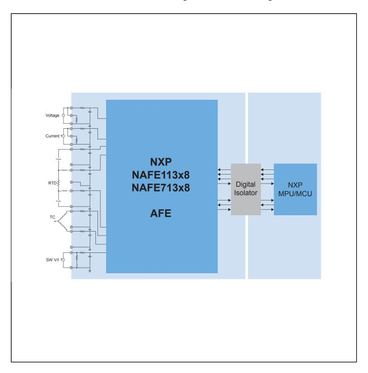
View additional information for Highly Configurable 8 Channel ±25 V Universal Input Analog Front-End.
