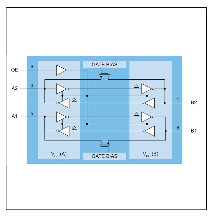
View additional information for Dual-Supply Translating Transceiver (Open-Drain, Auto-Direction Sensing).
