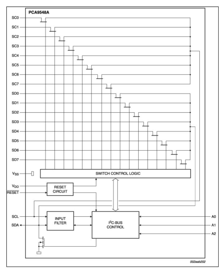
View additional information for Eight-Channel I<sup>2</sup>C-Bus Switch with Reset.
