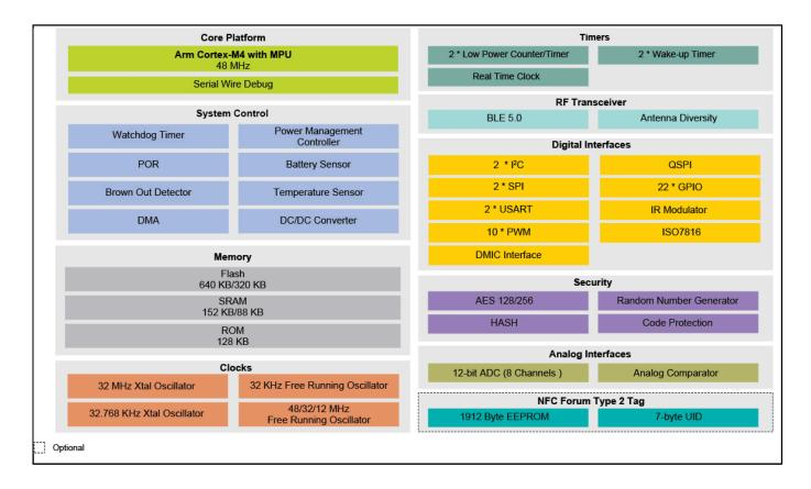
View additional information for QN9090/30: Bluetooth Low-Energy MCU with Arm®Cortex®-M4 CPU, Energy Efficiency, Analog and Digital Peripherals and NFC Tag Option.
