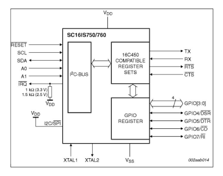
View additional information for Single UART with I<sup>2</sup>C-Bus/SPI Interface, 64 Bs of Transmit and Receive FIFOs, IrDA SIR Built-In Support.
