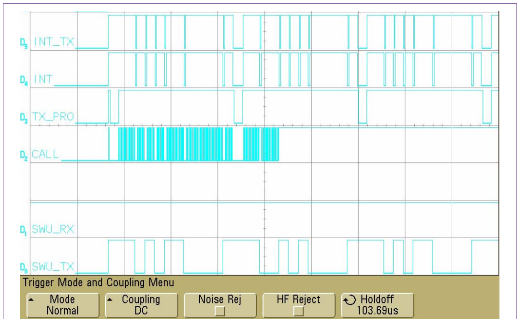
Fig 10. The Tx FIFO is larger than the whole greeting message (128 bytes vs. 122 bytes); Tx FIFO loading is interrupted by the software UART transmitter interrupt; individual interrupt servicing does not depend on the FIFO size
