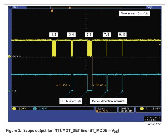
In BT\_MODE =  $V_{DD}$ , DRDY interrupt and motion detection interrupt pulse width = 5 ms ( $T_{PULSE-MOT}$  (typ)). The current interrupt pulse will be terminated when the device undergoes Active-Standby-Active transition before the pulse completion and thus may not span for entire 5 ms ( $T_{PULSE-MOT}$  (typ)).
