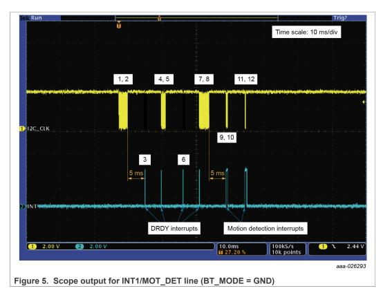
Self-test procedure for FXLS896xAF and FXLS897xCF accelerometer family
