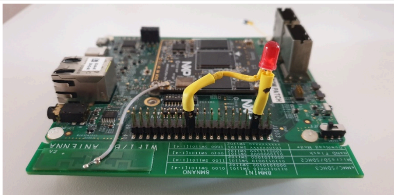
Figure 9. LED connected to GPIO5_IO13
