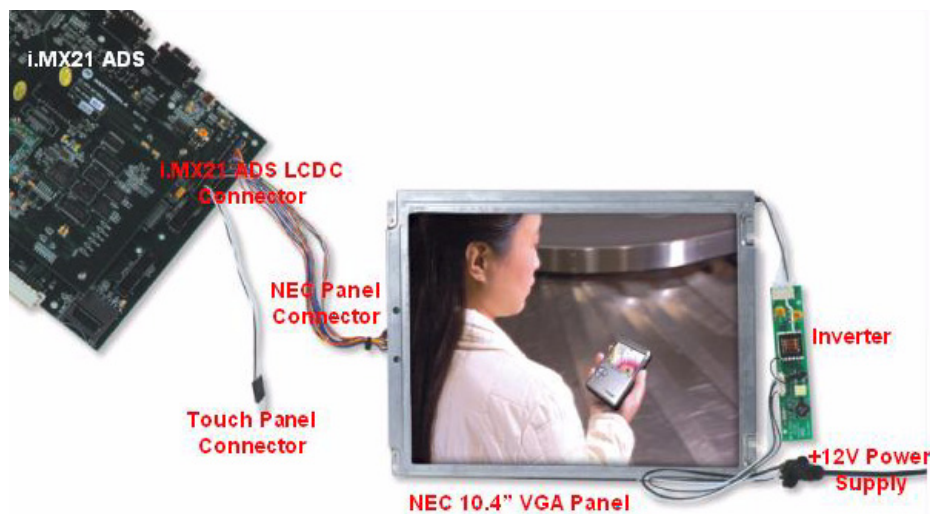
Figure 7. i.MX21 ADS and NEC VGA Panel Setup
