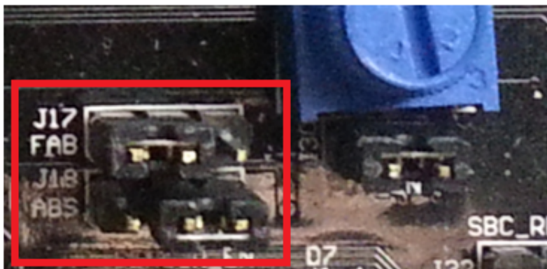
Figure 51. Jumper setting for Flash
