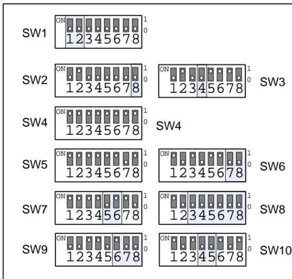
66 SYSCLK / 533 CCB (Platform) / 533 Core 0 & 800 Core 1, 933 DDR
