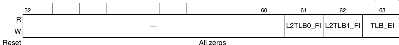
Figure 2-29. MMU Control and Status 0 (MMUCSR0) register
