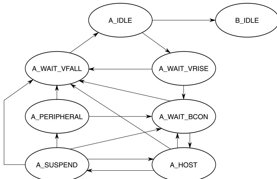
**Figure 40-93. Dual role A device flow diagram**
