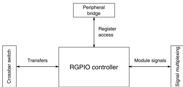
**Figure 3-45. RGPIo configuration**
