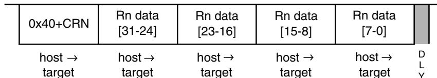
If the processor is halted, this command writes the 32-bit operand to the selected CPU general-purpose register (An, Dn). See [Table 51-39](#) for the CRN details when CRG is 01.
