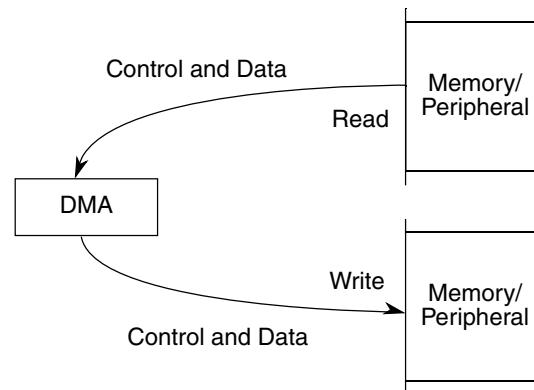
**Figure 20-2. Dual-Address Transfer**
