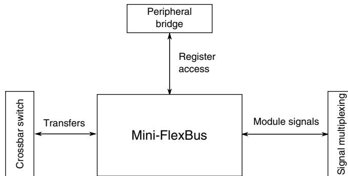
**Figure 3-21. Mini-FlexBus configuration**
