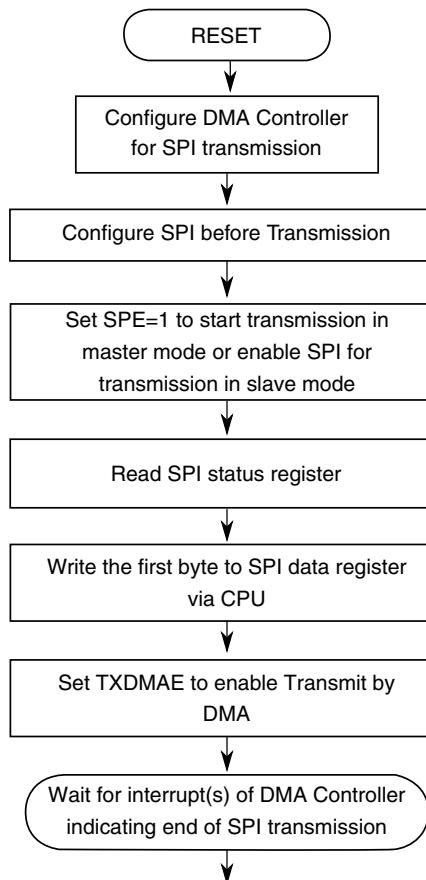
**Figure 39-37. Recommended startup of SPI transmit by DMA**
