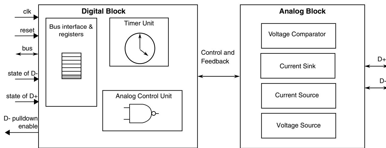
**Figure 41-1. Block diagram**
