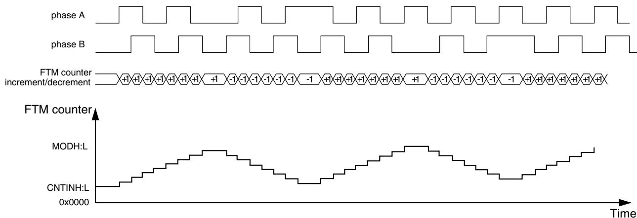
**Figure 38-218. Quadrature Decoder – Phase A and Phase B Encoding Mode**
