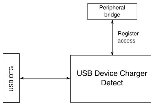
**Figure 3-39. USBDCD configuration**
