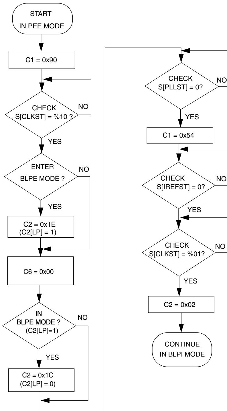
Figure 21-14. Flowchart of PEE to BLPI mode transition using a 4 MHz crystal
