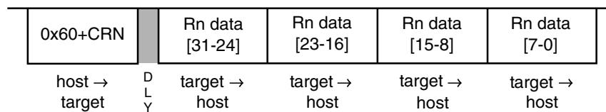
If the processor is halted, this command reads the selected CPU general-purpose register (An, Dn) and returns the 32-bit result. See [Table 51-39](#) for the CRN details when CRG is 01.
