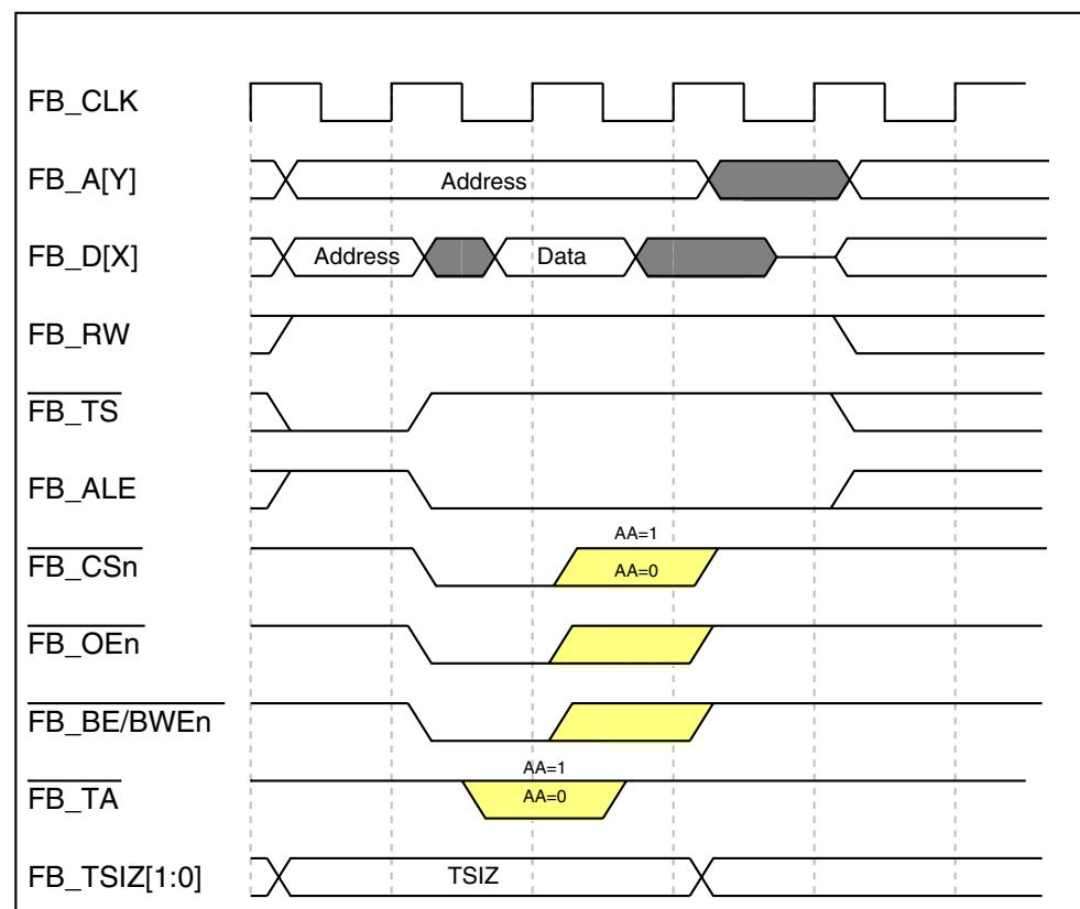
Figure 25-21. Basic Read-Bus Cycle (No Wait States)
