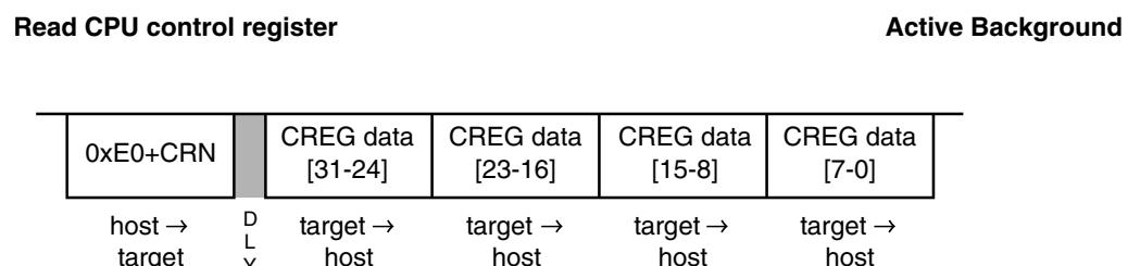
If the processor is halted, this command reads the selected control register and returns the 32-bit result. This register grouping includes the PC, SR, CPUCR, MACSR, MASK, ACC, VBR, and OTHER\_A7. Accesses to processor control registers are always 32-bits wide, regardless of implemented register width. The register is addressed through the core register number (CRN). See [Table 51-39](#) for the CRN details when CRG is 11.
