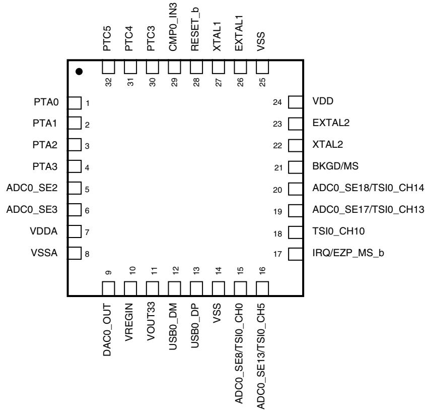
**Figure 9-5. 32-pin QFN**
