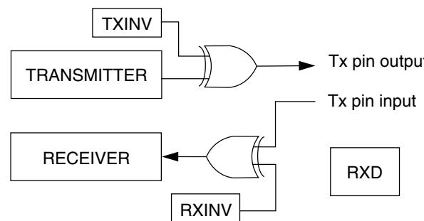
**Figure 44-114. Single-wire operation (C1[LOOPS] = 1, C1[RSRC] = 1)**
