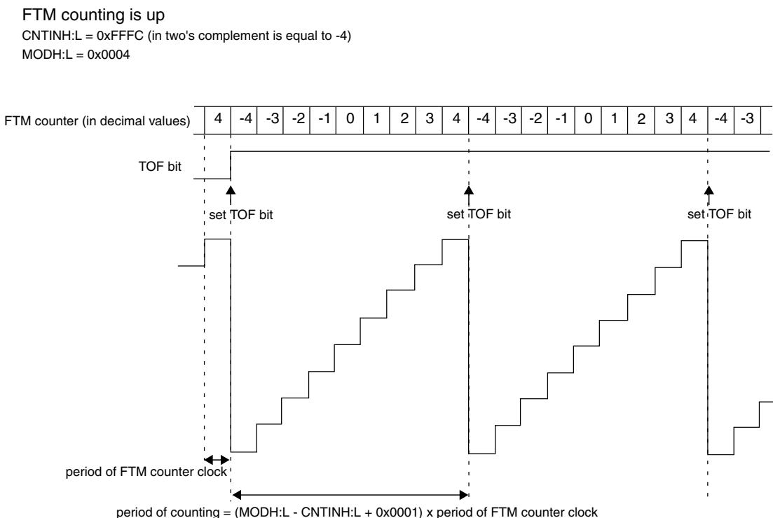
**Figure 38-145. Example of FTM up and signed counting**
