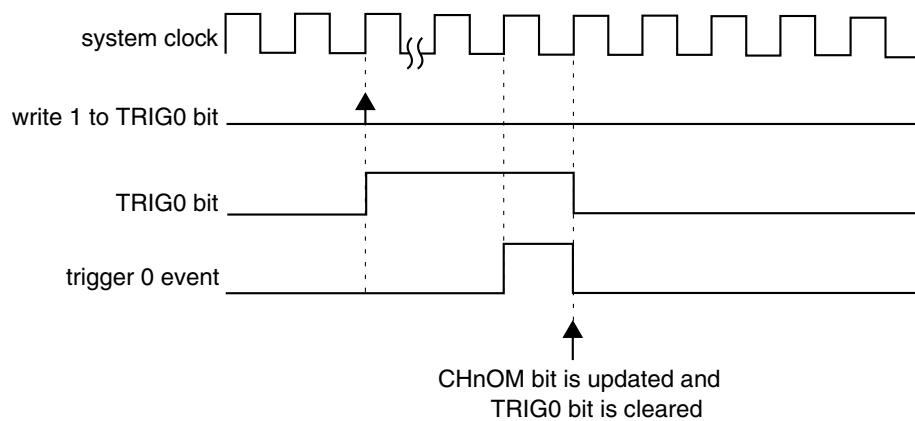
**Figure 38-189. CHnOM synchronization when (SYNCHOM = 1), (PWMSYNC = 0), and a hardware trigger was used**
