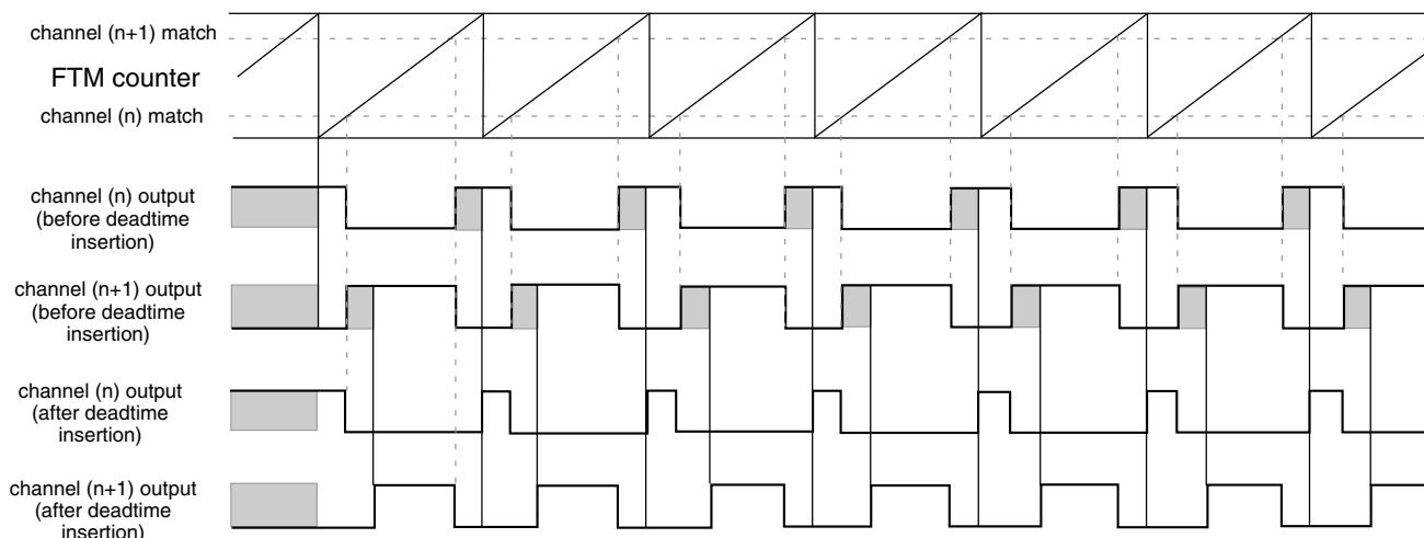
**Figure 38-195. Deadtime insertion with  $\text{ELSnB:ELSnA} = X:1$ ,  $\text{POL}(n) = 0$ , and  $\text{POL}(n+1) = 0$**
