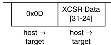
Write the special status byte of XCSR (XCSR[31–24]). This command can be executed in any mode.
