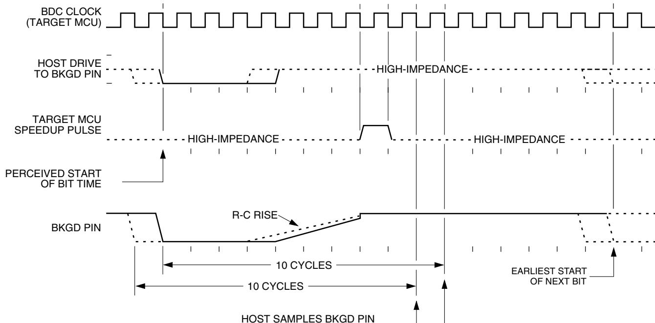
**Figure 51-4. BDC Target-to-Host Serial Bit Timing (Logic 1)**
