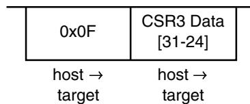
Write the most significant byte of CSR3 (CSR3[31–24]). This command can be executed in any mode.
