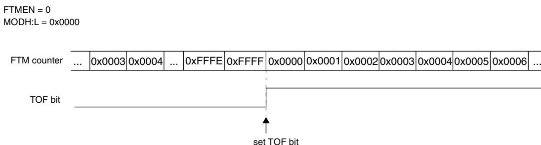
**Figure 38-149. Example when the FTM counter is a free running**
