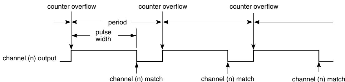
**Figure 38-156. EPWM period and pulse width with ELSnB:ELSnA = 1:0**
