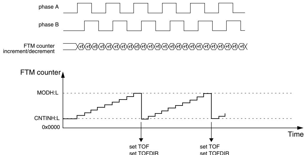
**Figure 38-219. FTM Counter Overflow in Up Counting for Quadrature Decoder Mode**
