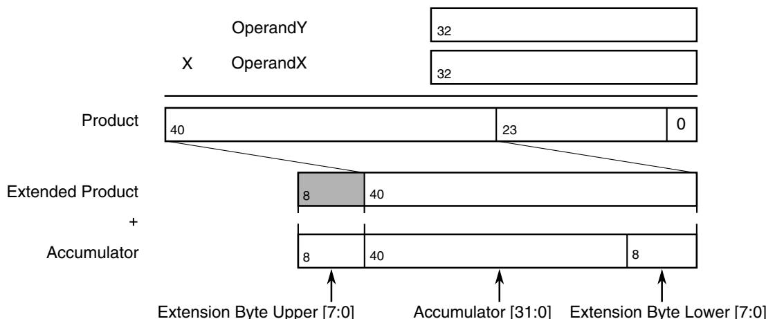
**Figure 12-2. Fractional Alignment**
