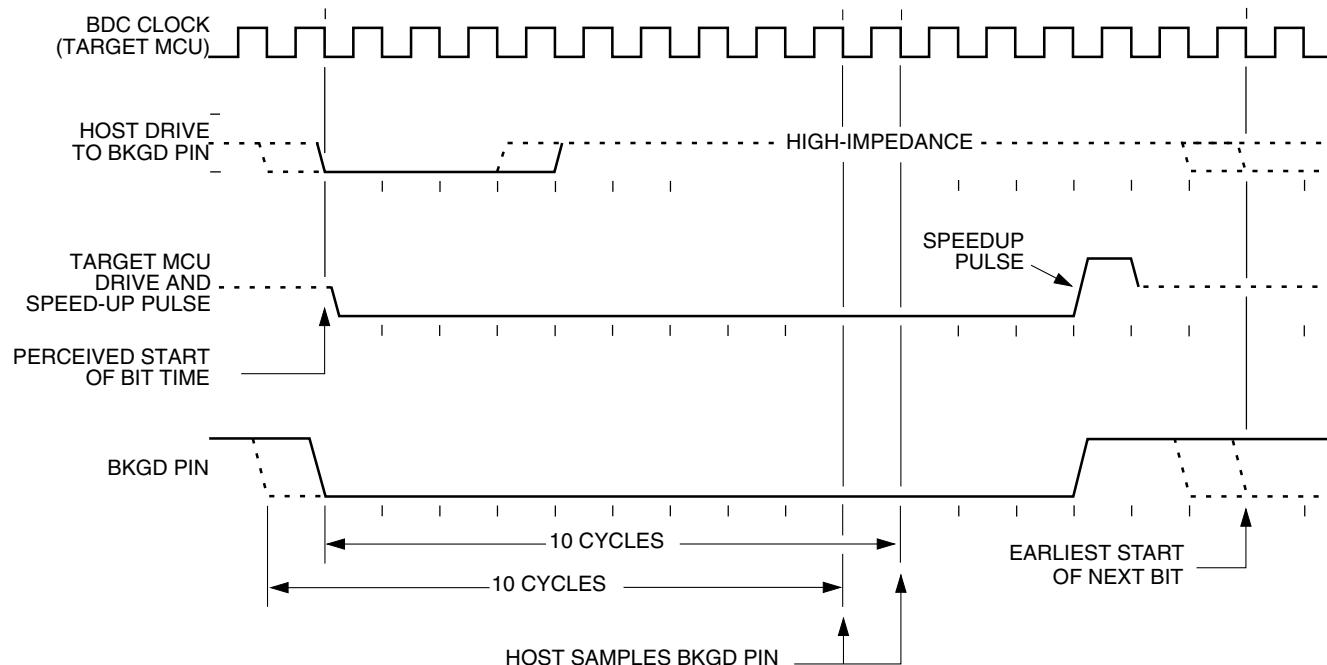
Figure 51-5. BDM Target-to-Host Serial Bit Timing (Logic 0)
