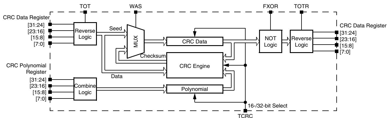
**Figure 29-1. Programmable cyclic redundancy check (CRC) block diagram**
