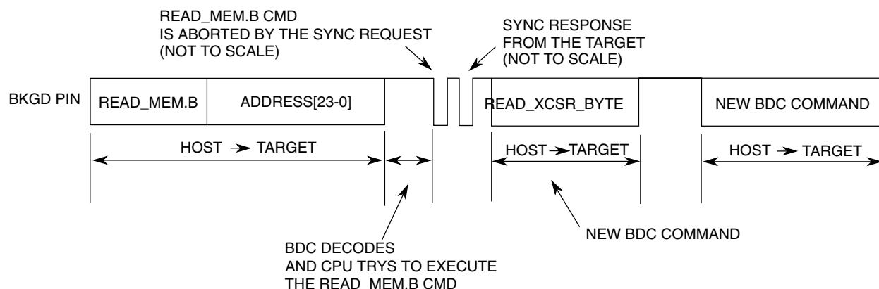
**Figure 51-9. ACK Abort Procedure at the Command Level**
