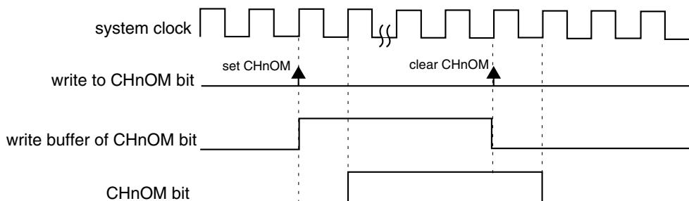
**Figure 38-187. CHnOM synchronization when (SYNCHOM = 0)**
