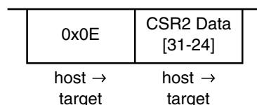
Write the most significant byte of CSR2 (CSR2[31–24]). This command can be executed in any mode.
