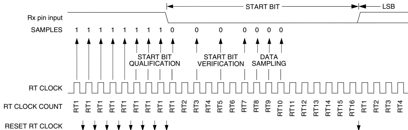
**Figure 44-94. Receiver data sampling**
