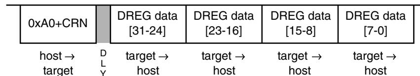
This command reads the selected debug control register and returns the 32-bit result. This register grouping includes the CSR, XCSR, CSR2, and CSR3. Accesses to debug control registers are always 32-bits wide, regardless of implemented register width. The register is addressed through the core register number (CRN). See [Table 51-4](#) for CRN details.
