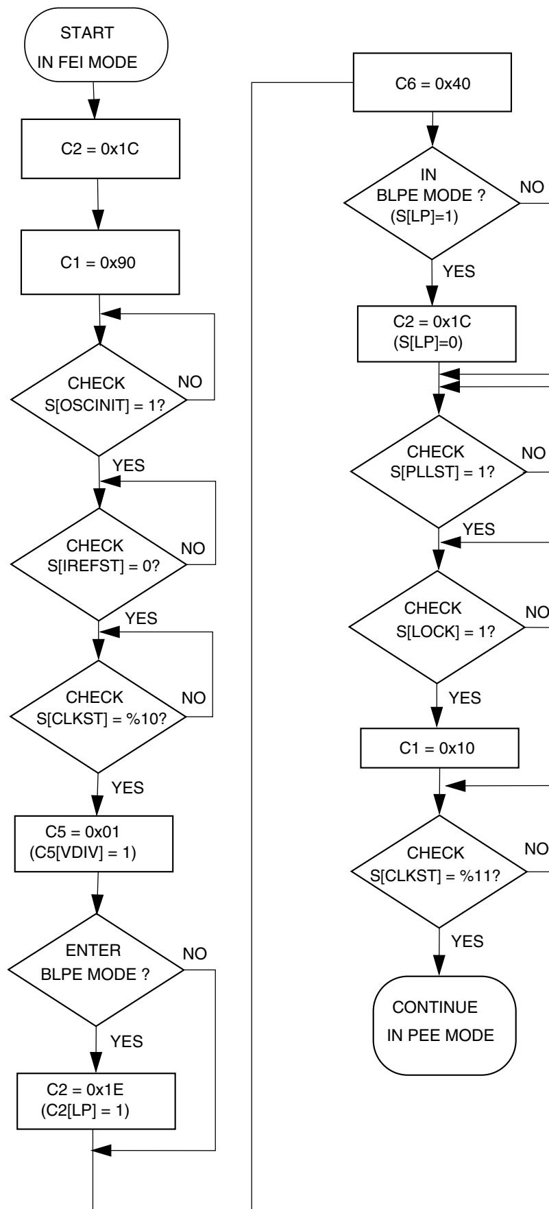
**Figure 21-13. Flowchart of FEI to PEE mode transition using an 4 MHz crystal**
