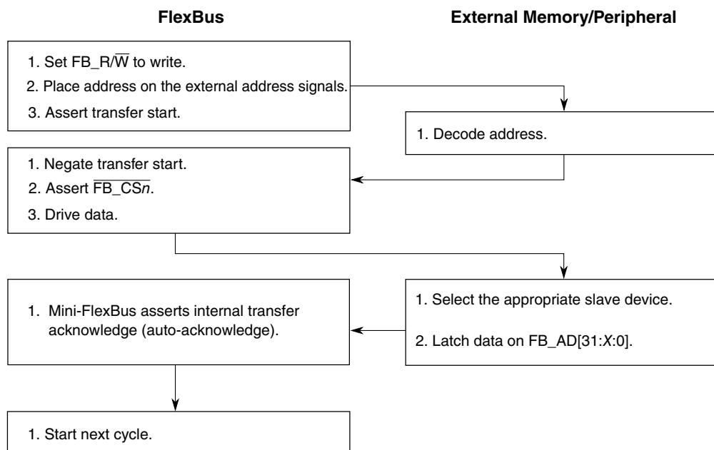
**Figure 25-15. Write-Cycle Flowchart**
