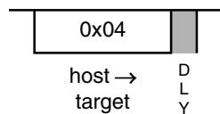
Provided XCSR[ENBDM] is set (BDM enabled), the BACKGROUND command causes the target MCU to enter active background (halt) mode as soon as the current CPU instruction finishes. If ENBDM is cleared (its default value), the BACKGROUND command is ignored.
