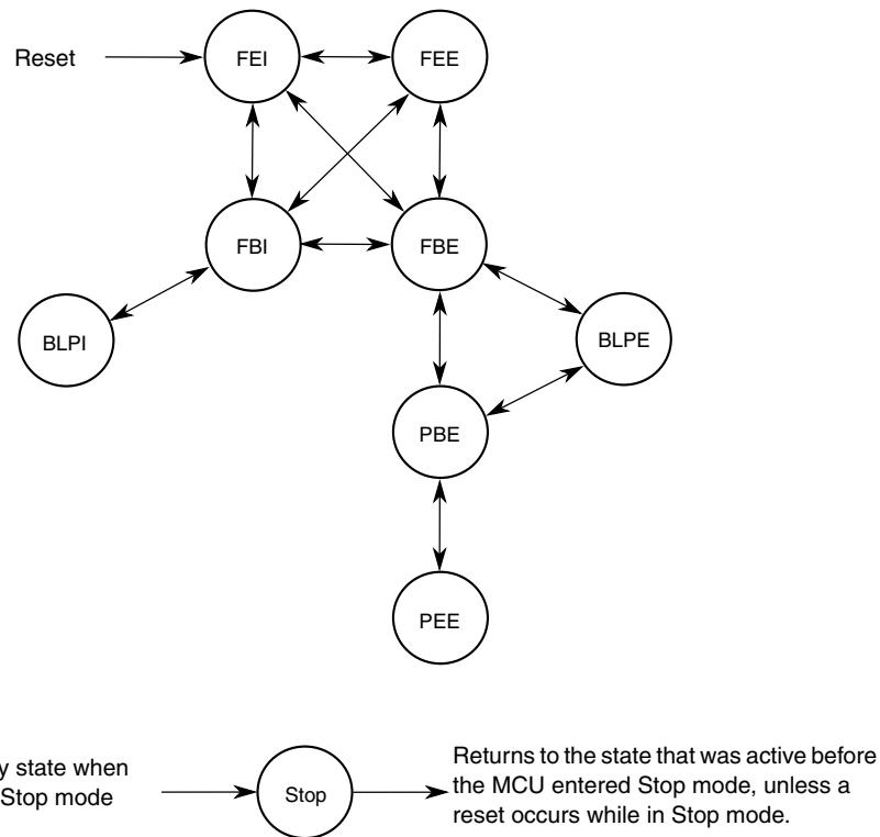
**Figure 21-12. MCG mode state diagram**
