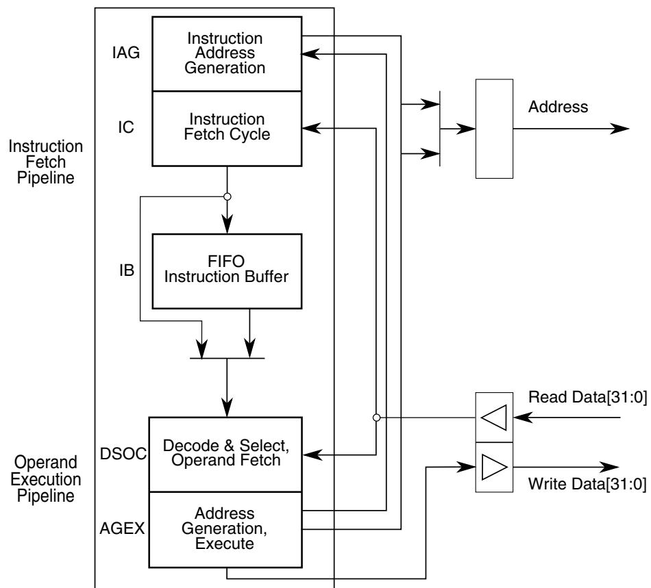
**Figure 11-1. V1 ColdFire Core Pipelines**
