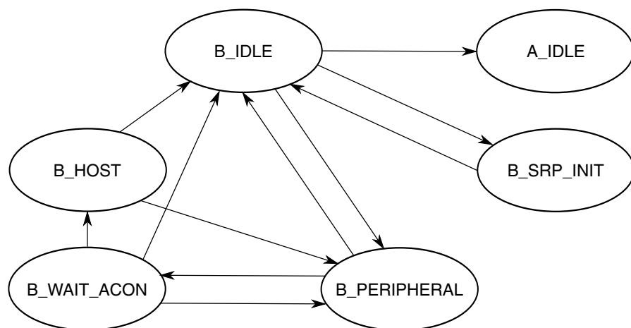
**Figure 40-94. Dual role B device flow diagram****Table 40-97. State descriptions for the dual role B device flow**
