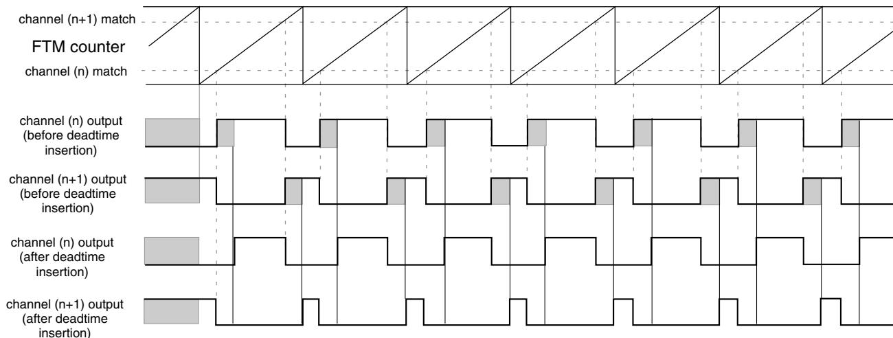
**Figure 38-194. Deadtime insertion with  $\text{ELSnB:ELSnA} = 1:0$ ,  $\text{POL}(n) = 0$ , and  $\text{POL}(n+1) = 0$**
