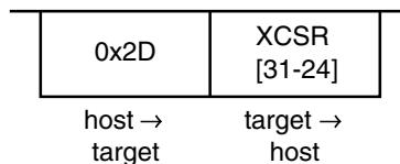
Read the special status byte of XCSR (XCSR[31–24]). This command can be executed in any mode.
