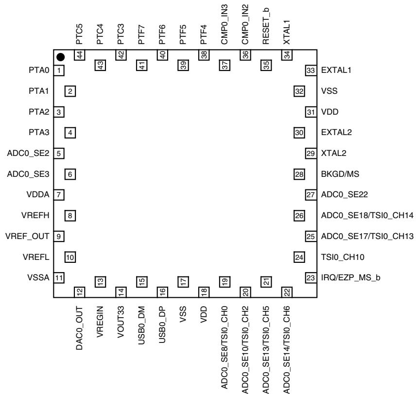
**Figure 9-4. 44-pin Laminate QFN**
