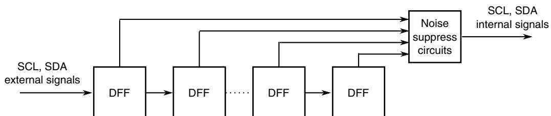
**Figure 43-65. Programmable input glitch filter diagram**
