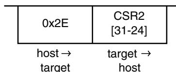
Read the most significant byte of CSR2 (CSR2[31–24]). This command can be executed in any mode.
