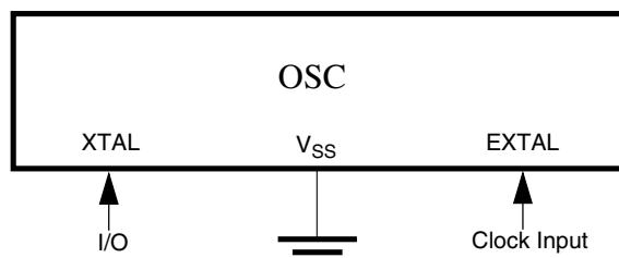
Figure 22-6. External Clock Connections
