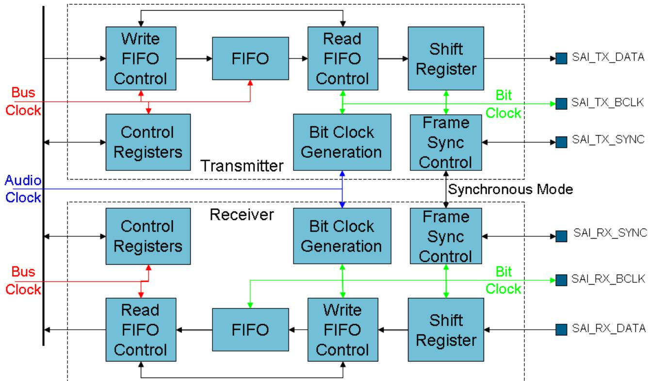
**Figure 45-1. I<sup>2</sup>S/SAI block diagram**
