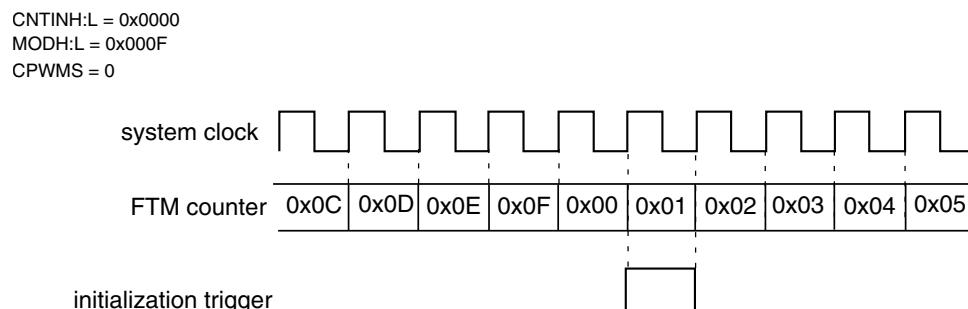
Figure 38-205. Initialization trigger is generated when the FTM counter achieves the value of CNTINH:L
