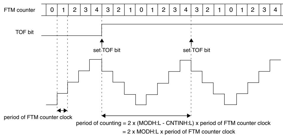
**Figure 38-148. Example of up-down counting when CNTIN = 0x0000**
