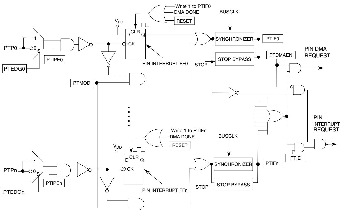
**Figure 47-81. Diagram of pin interrupt function**
