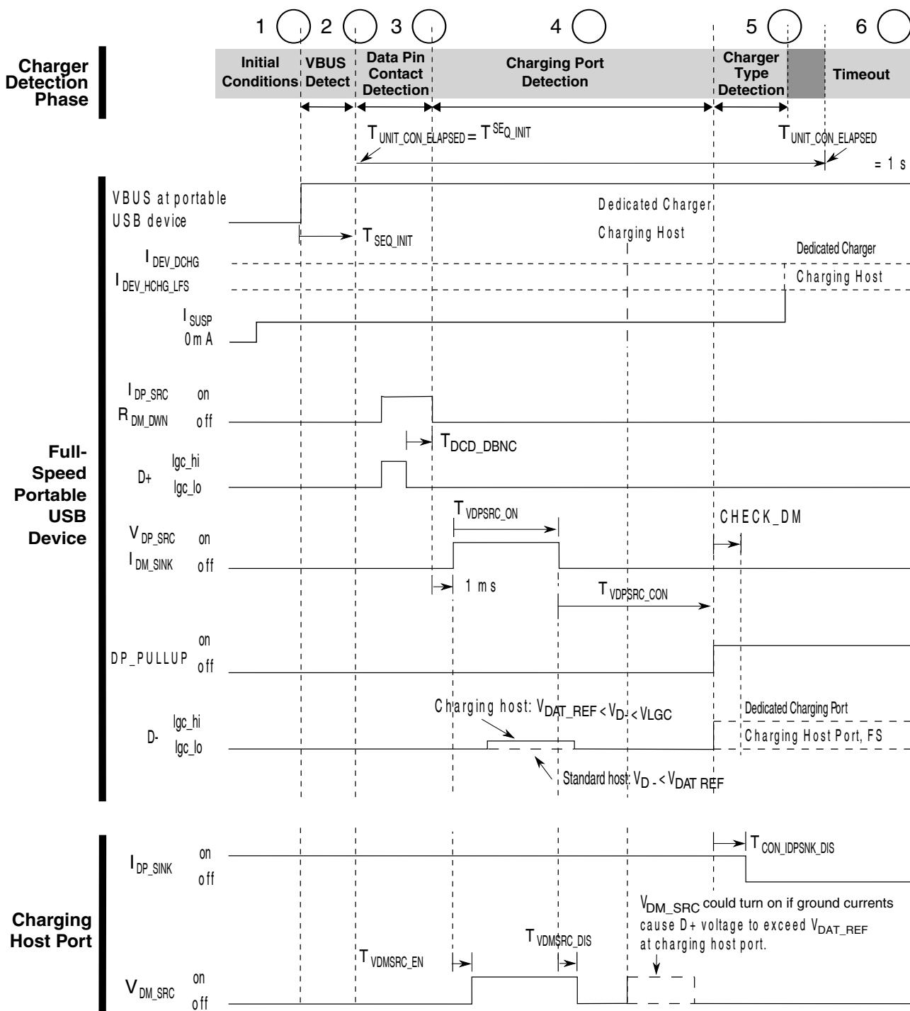
Figure 41-9. Full speed charger detection timing
