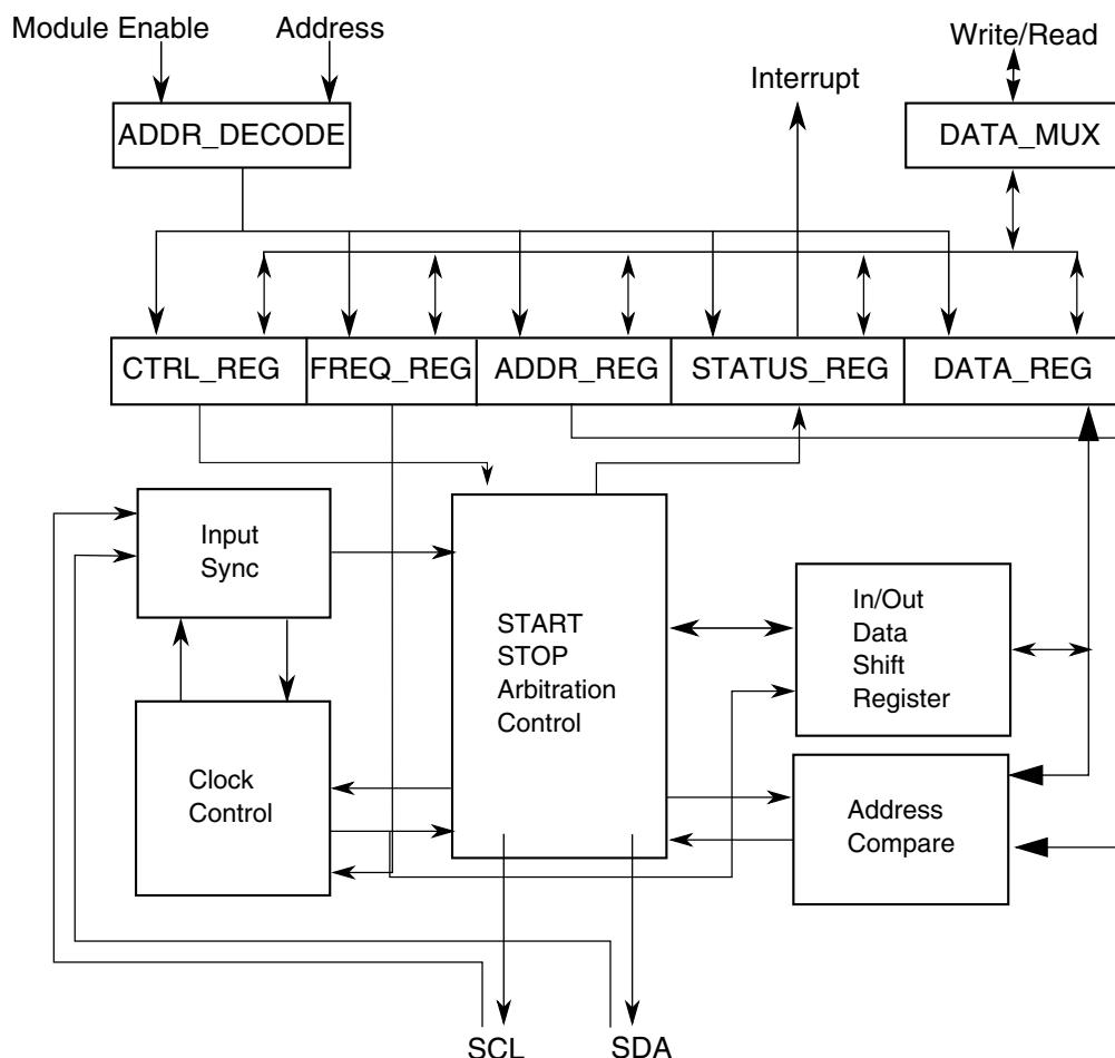
**Figure 43-1. I<sup>2</sup>C Functional block diagram**
