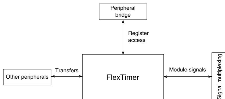
**Figure 3-30. FlexTimer configuration**
