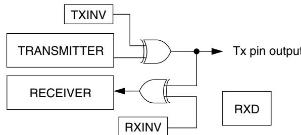
**Figure 44-115. Loop operation ( $C1[LOOPS] = 1$ ,  $C1[RSRC] = 0$ )**
