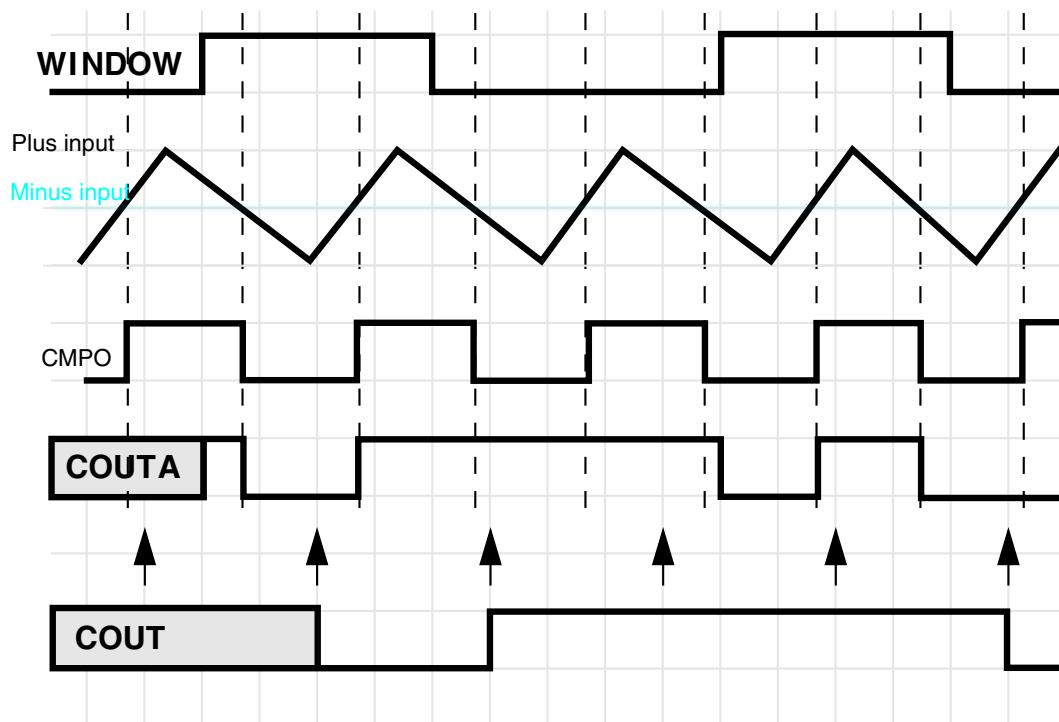
**Figure 31-22. Windowed/resampled mode operation**
