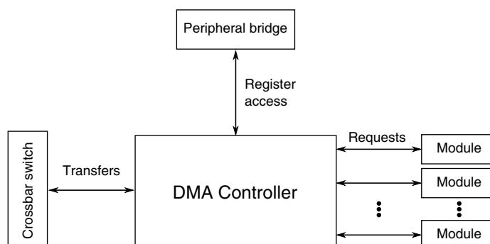
**Figure 3-5. DMA Controller configuration****Table 3-7. Reference links to related information**
