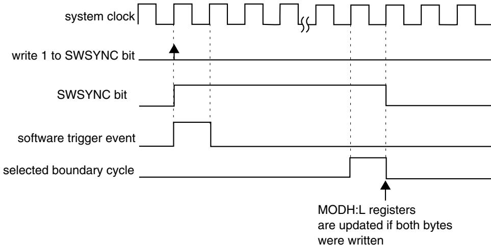
**Figure 38-186. MODH:L synchronization when (PWMSYNC = 1)**
