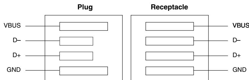
**Figure 41-10. Relative pin positions in USB plugs and receptacles**
