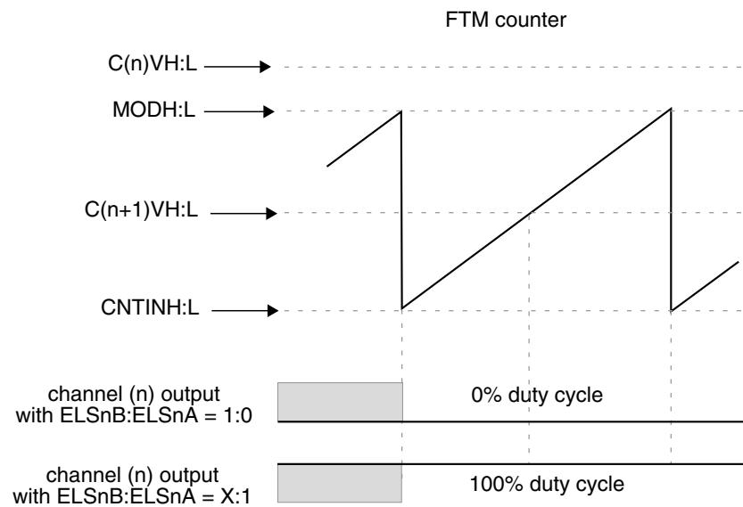
**Figure 38-175. Channel (n) output if ( $C(n)V > MOD$ ) and ( $CNTIN < C(n)V < MOD$ )**
