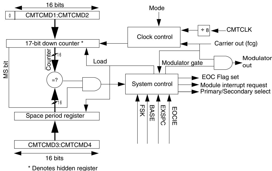
**Figure 37-16. Modulator block diagram**
