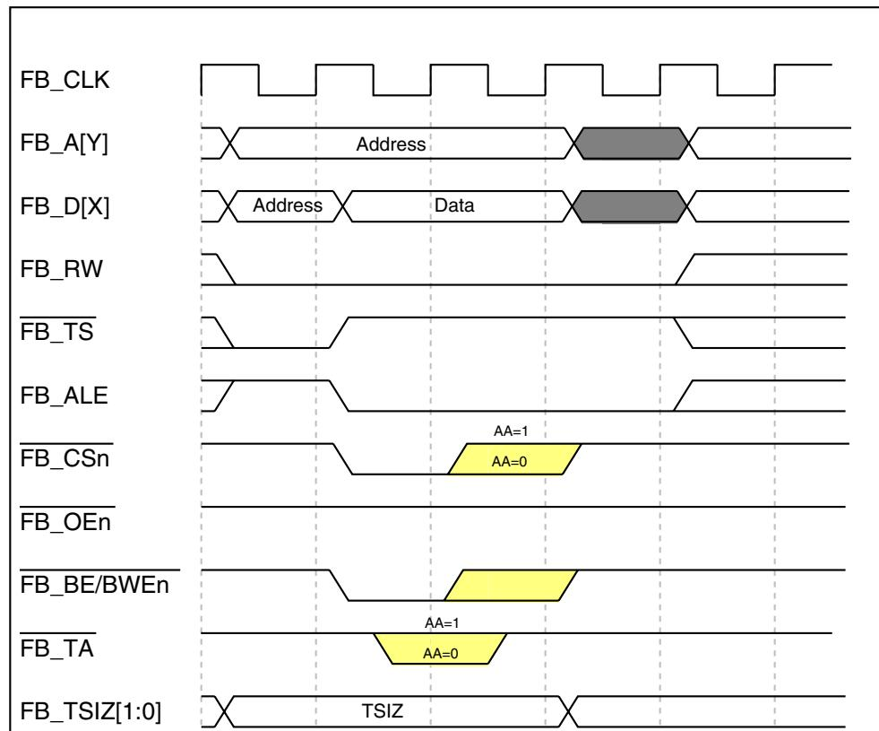
**Figure 25-16. Basic Write-Bus Cycle**
