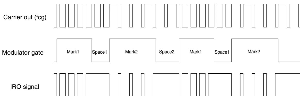
**Figure 37-18. Example: CMT output in FSK mode**
