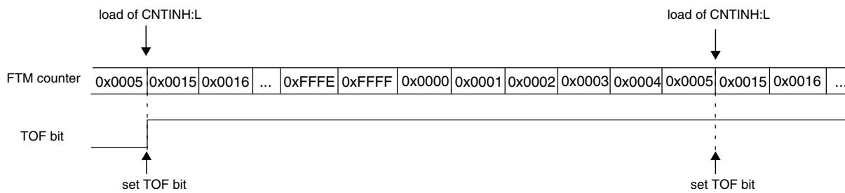
**Figure 38-147. Example of up counting when the value of CNTIN registers is greater than the value of MOD registers**
