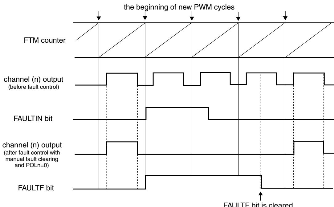
**Figure 38-202. Fault control with manual fault clearing**
