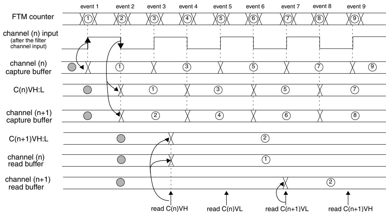
**Figure 38-215. Dual edge capture mode read coherency mechanism**
