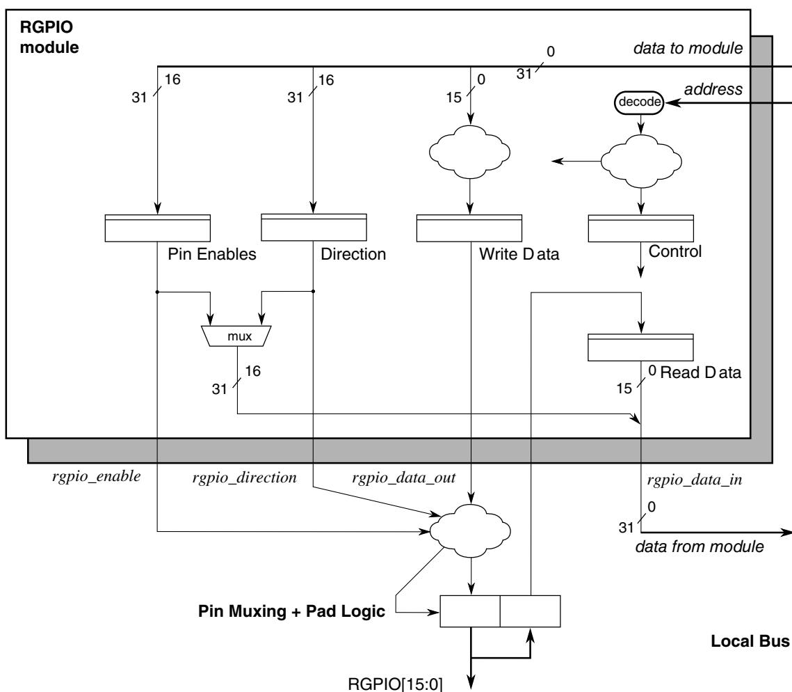
**Figure 46-1. RGPIO Block Diagram**
