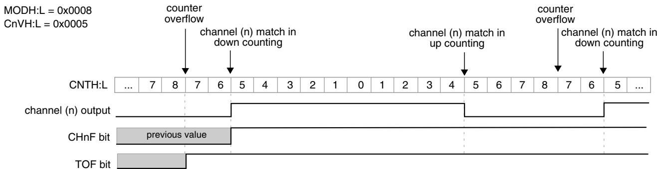
**Figure 38-160. CPWM signal with  $\text{ELSnB:ELSnA} = 1:0$**
