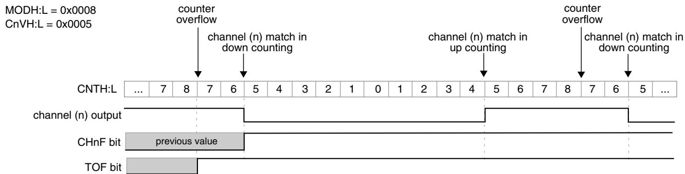
**Figure 38-161. CPWM signal with  $\text{ELSnB:ELSnA} = X:1$**
