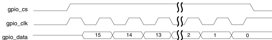
**Figure 46-10. GPIO SPI Example Timing Diagram**
