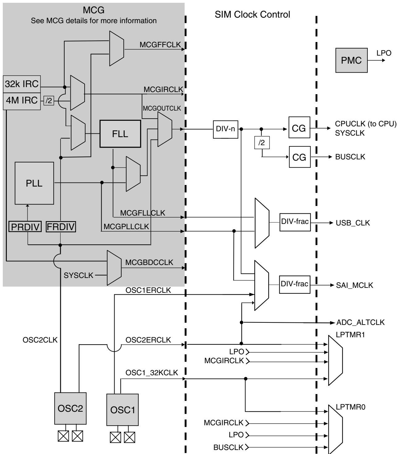
Figure 5-1. Clocking diagram
