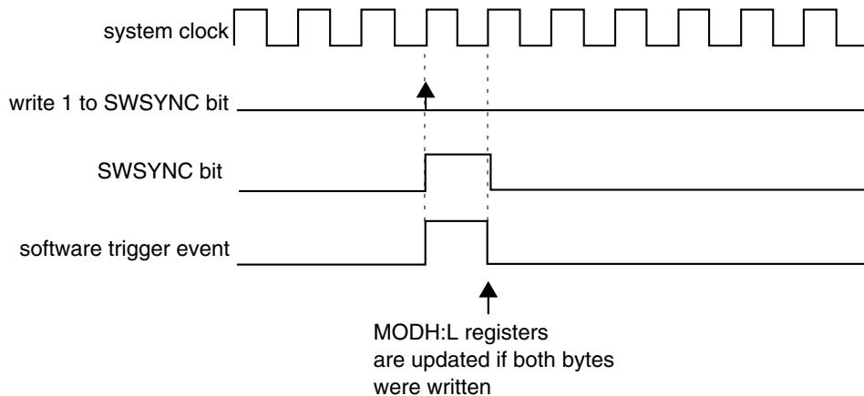
**Figure 38-184. MODH:L synchronization when (PWMSYNC = 0), (REINIT = 1), and software trigger was used**
