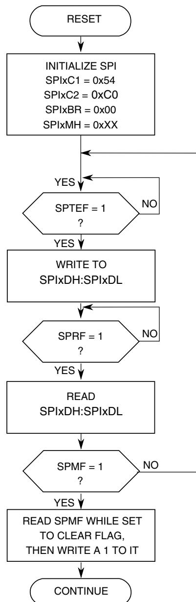
**Figure 39-41. Initialization Flowchart Example for SPI Master Device in 16-bit Mode for FIFOMODE = 0**
