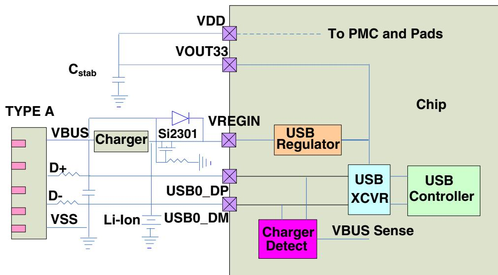
**Figure 3-36. USB regulator Li-ion use case**
