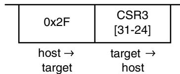
Read the most significant byte of the CSR3 (CSR3[31–24]). This command can be executed in any mode.
