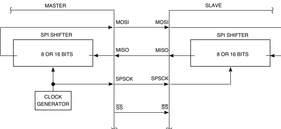
**Figure 39-1. SPI System Connections**
