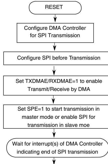
**Figure 39-36. Basic Flow of SPI Transmission by DMA**
