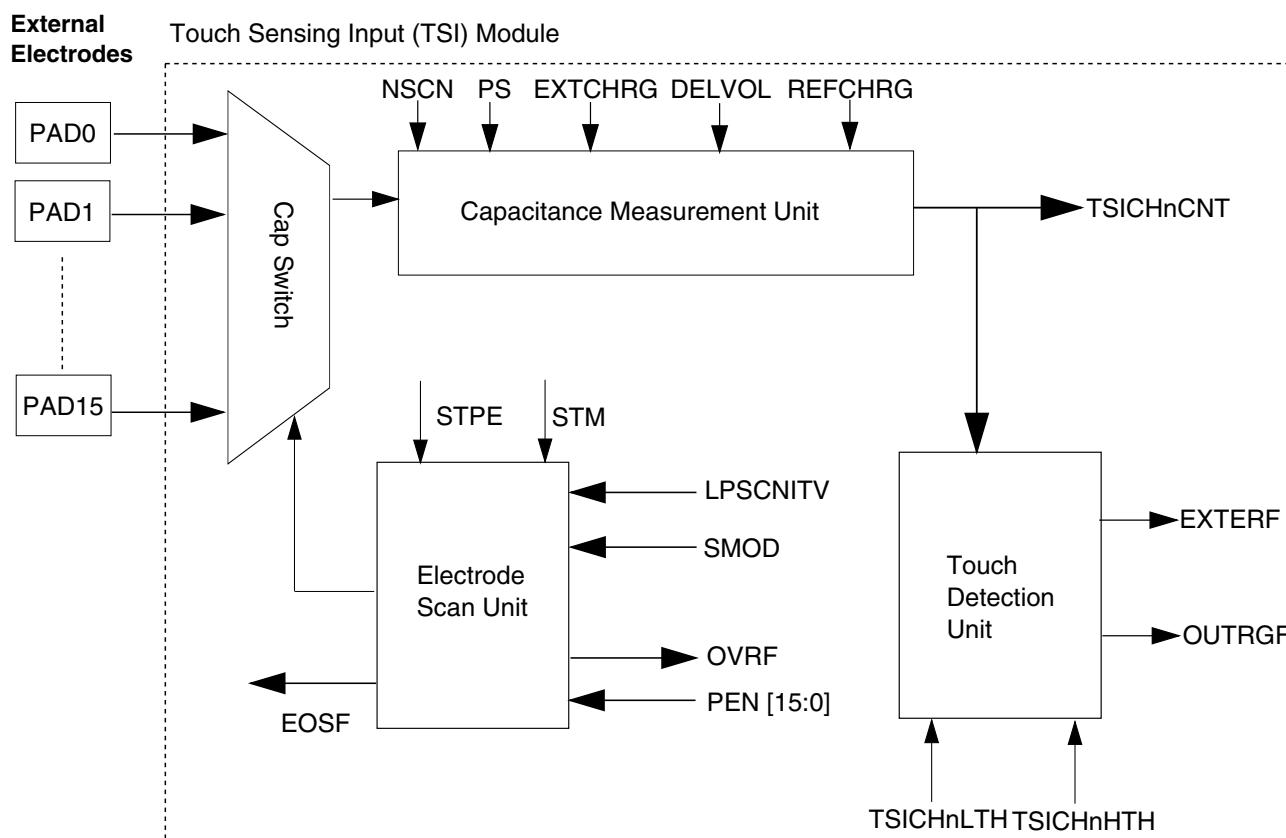
**Figure 49-1. Touch sensing input block diagram**
