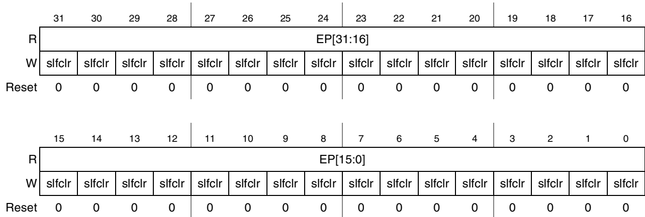
Figure 52-19. Channel Event Pending (EVTPEND) Register
