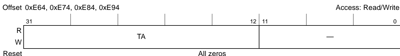
Figure 14-128. PCI Express RC Inbound Window Translation Address Register n (PEX_RCIWTAR0–PEX_RCIWTAR3)
