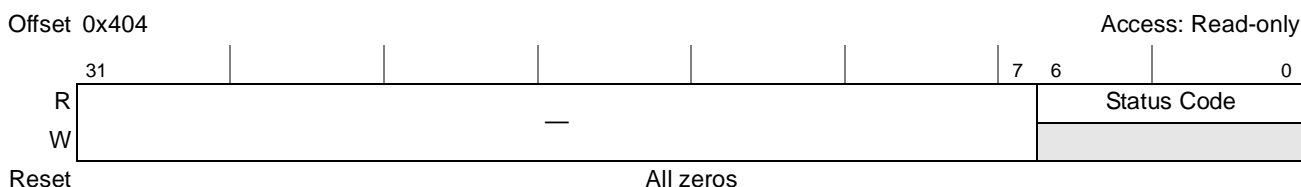
Figure 14-80. PCI Express LTSSM State Status Register (PEX_LTSSM_STAT)
