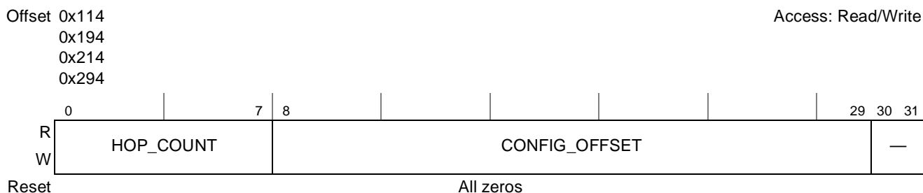
Figure 14-11. Source Address Registers for RapidIO Maintenance Reads (SAR n )
