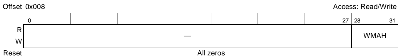
Figure 19-4. Watchpoint Monitor Address High Register (WMAHR)
