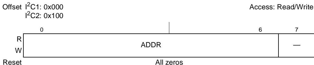
Figure 10-2. I 2 C Address Register (I2CADR)
