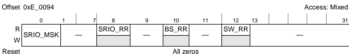
Figure 17-14. Reset Request Status and Control Register (RSTRSCR)
