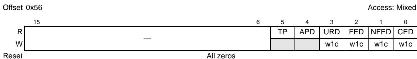
Figure 17-98. PCI Express Device Status Register
