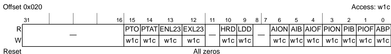
Figure 17-17. PCI Express PME and Message Detect Register (PEX_PME_MES_DR)
