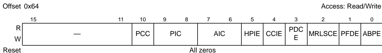
Figure 17-103. PCI Express Slot Control Register
