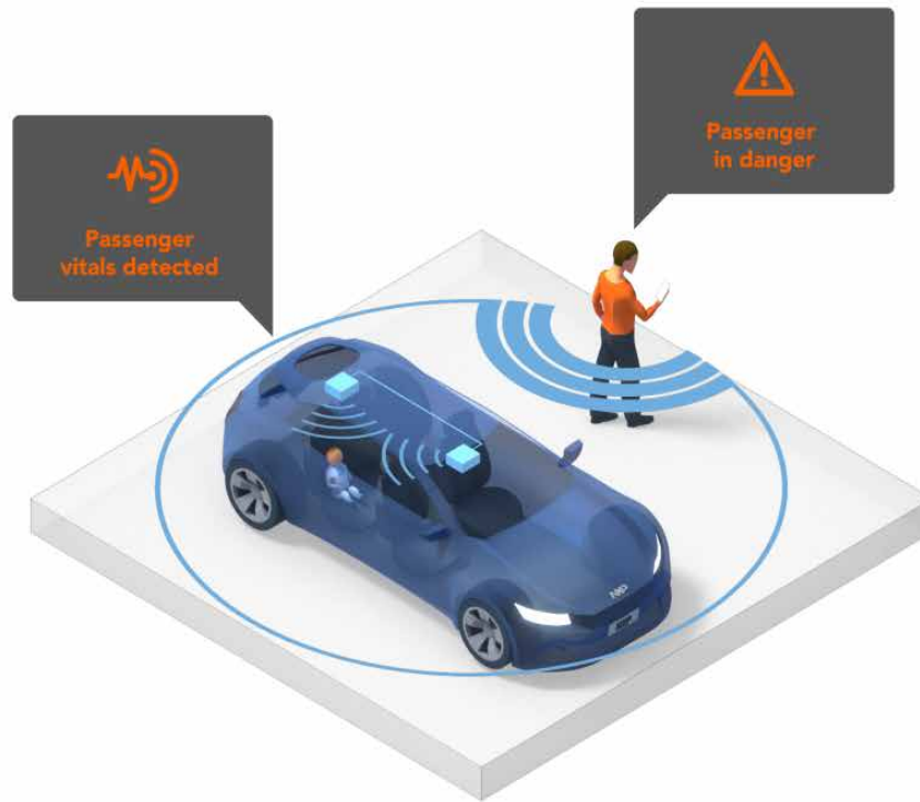
Figure 1: UWB Radar Child Presence Detection
